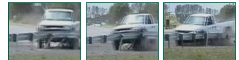
Test Level 3 crash test of NU-GUARD-27 design.
