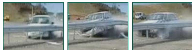
Test Level 3 crash test of NU-GUARD-31 design.
