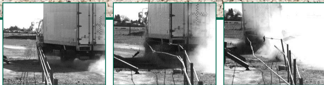
Test Level 4 "box truck" crash test of NU-CABLE TL-4 design.
